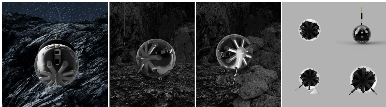
Fig. 1. The DAEDALUS sphere. From left to right: First, Daedalus sphere is descended into the pit by a crane. Second, DAEDALUS in scanning mode. Third, Different modes of DAEDALUS. Fourth, DAEDALUS overcoming obstacles by pushing with its rods.
